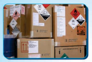
U.N. Certified Packaging which are tested and approved by appropriated national authorities must be used for all forms of Transport Packing Performance established by a variety of tests which can include pressure, drop and stack testing.
